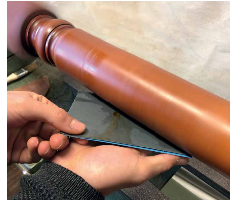
▲ The dust in the wet and dry combines with the oil to form a polishing slurry.
