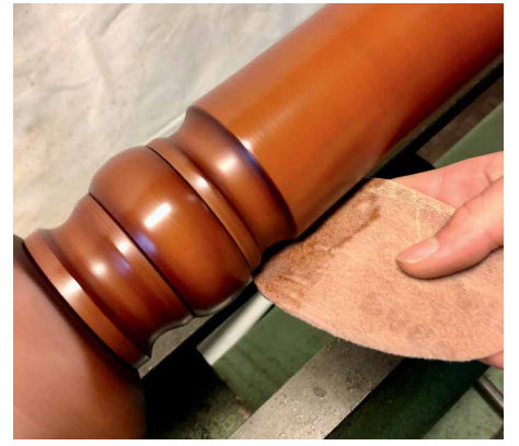
▲ Working the now dry surface with 1200-2000 wet and dry can produce a mirror finish.
