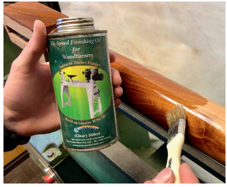
▲ Hi-Speed Finishing Oil is easy to apply. Two liberal coats, a couple of hours apart, is all it takes.
